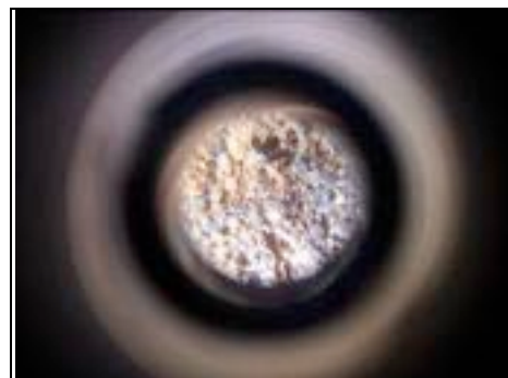
Microscope photo of the brickwork indicating salts discharging down the walls meaning the gutters / roofs are not working properly
